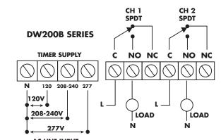
AC LINE INPUT SELECT PROPER TERMINALS AND APPLY ONLY ONE VOLTAGE
