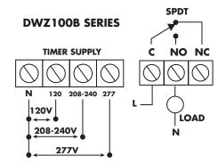
AC LINE INPUT SELECT PROPER TERMINALS AND APPLY ONLY ONE VOLTAGE
