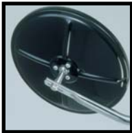
All mirrors come with an adjustable ball and swivel.
