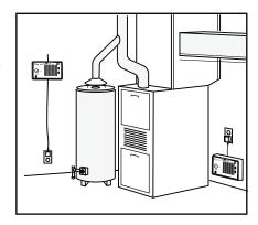
PROPANE GAS To detect Propane Gas place the alarm low -Propane Gas sinks.
