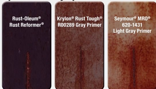
Rust-Oleum® Rust Reformer® vs Enamel Primers Direct-to-rusted metal and exposed to salt spray for 310 hours
