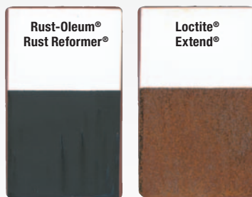
Rust-Oleum® Rust Reformer® vs Loctite® Extend® Bare rusted steel panels coated with rust converter and exposed to salt spray for less than a week
