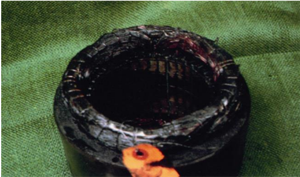
Windings from a severe burnout
