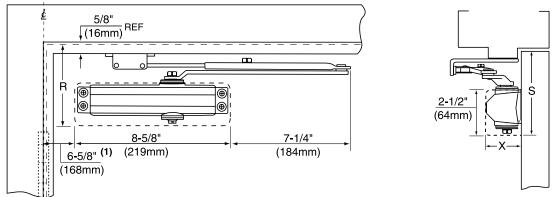
Center to center of mounting holes is: 8" (203mm) horizontally x 3/4" (19mm) vertically
