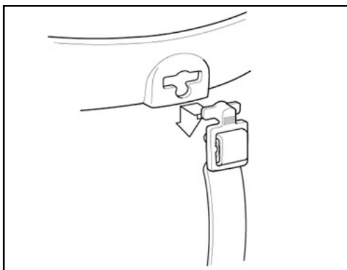
Fig. 16: Installing the Chin Strap
