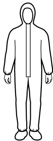
Bound Seam Coverall, storm flap over zipper, attached hood, boots, elastic wrists.
