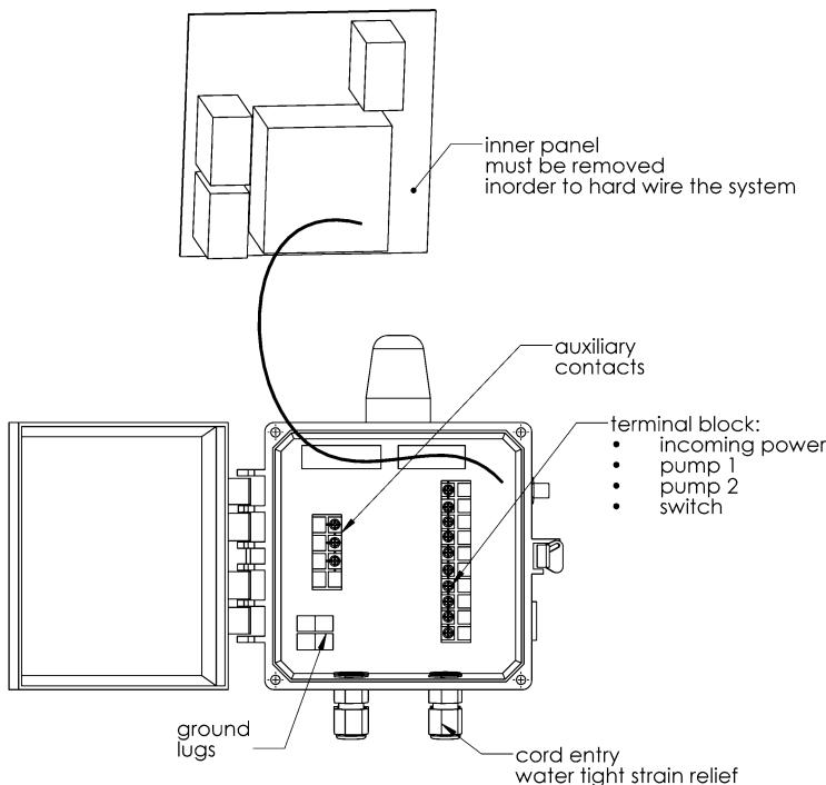
Models: PDCW-115 and PDCW-230 require hard wiring, the inner panel must be removed to provide access to the terminal block(s) inside the panel. The plug of the pumps and switch must be cut off and wires stripped. Feed the cords, along with the incoming power, through the water tight strain relief bushings and wire into the terminal block mounted in the PDC panel. A wiring schematic is provided beside the terminal block. The panel has a secondary terminal block for auxiliary contacts if required.
