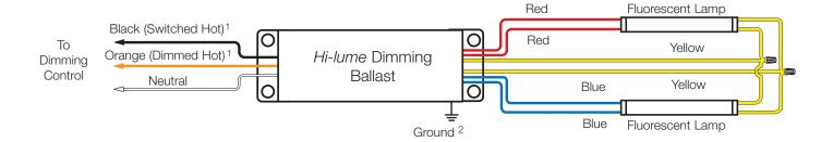
Note: For T5-HO lamps, maximum lamp-to-ballast wire length is 7 feet (2 m).
