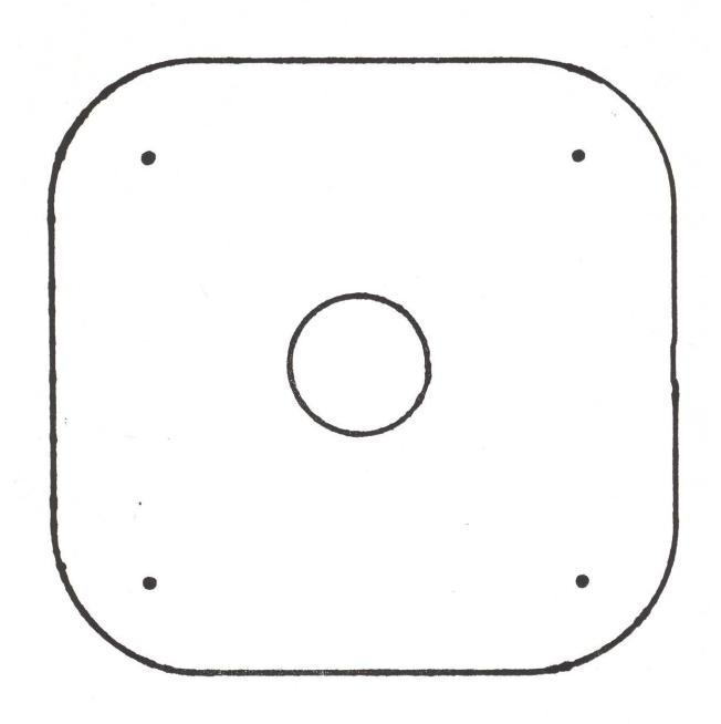
Dimensions of the footprint: 5.75" X 5.75" The installation holes are on 4" centers
