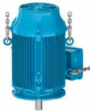
Figure 4.11 - End result: motor placed in vertical position
