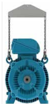
Figure 4.6 - Use of a spreader bar for lifting
