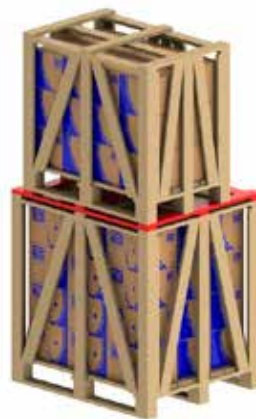
Figure 5.5 - Use of additional battens for stacking
