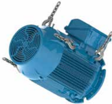
Figure 4.18 - Motor is being rotated to horizontal position
