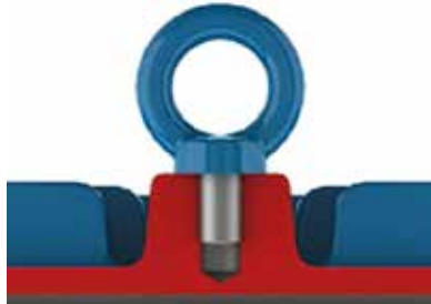
Figure 4.1 - Correct tightening of the eyebolt
