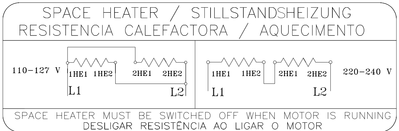
Figure 6.17 - Dual voltage space heater connection
