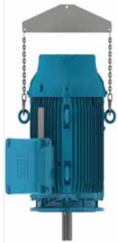
Figure 4.7 - Lifting of vertical mounted motors
