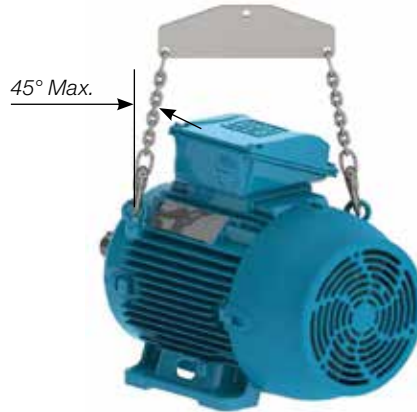
Figure 4.4 - Maximum resulting angle for motors with two or more lifting eyebolts
