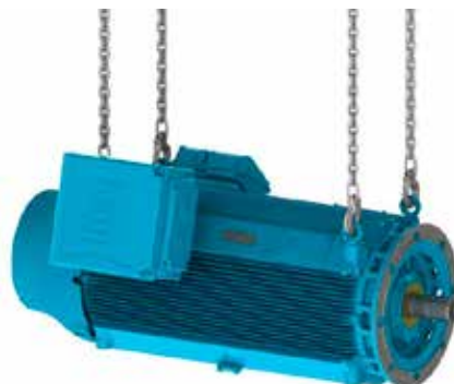
Figure 4.12 - Lifting HGF motor with two hoists
