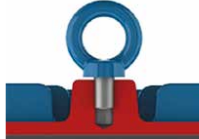
Figure 4.2 - Incorrect tightening of the eyebolt
