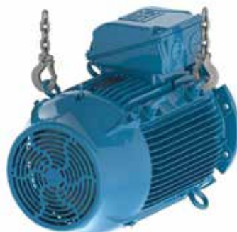
Figure 4.19 - Final result: motor placed in horizontal position
