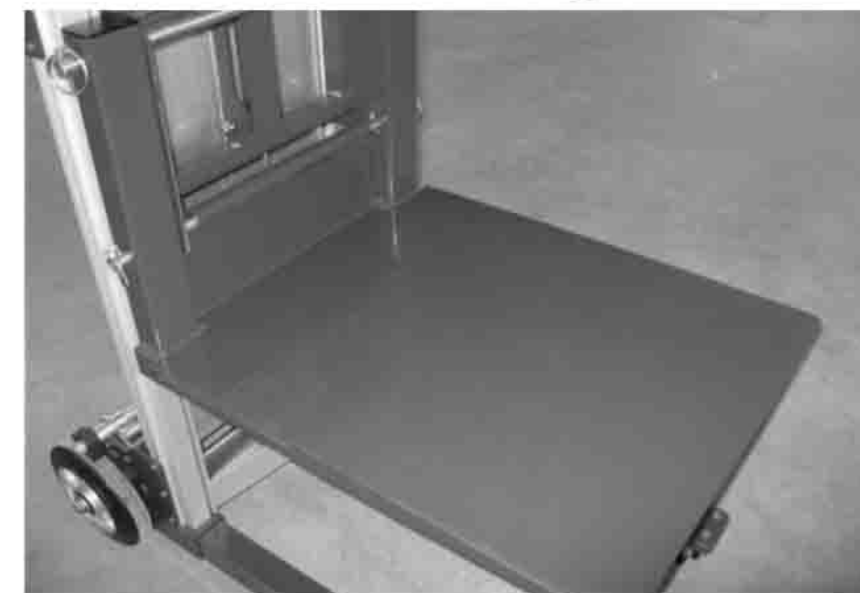
Set the connecting channel on top of the lower carriage cross bar; let the deck rest on top of the forks
