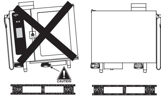
**NOTE:** To avoid equipment damage, observe attention label on oven for area to avoid with lifting fork.
