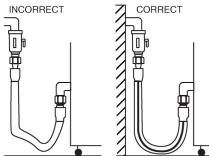
Gas piping used on gas connections must avoid sharp bends that may restrict the flow of gas to the appliance. If the connected pressure exceeds 14.0" W.C. (3.5 kPa), a step-down regulator is required to be supplied by the owner/operator.
