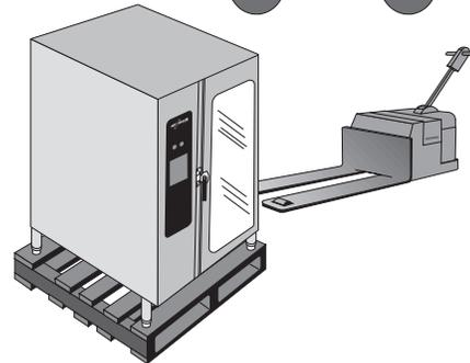
**NOTE:** Note dimensions required for doorways and aisles for access of the oven and pallet to the installation site. Transport the oven in an upright and level position only. Do not tilt the oven.
