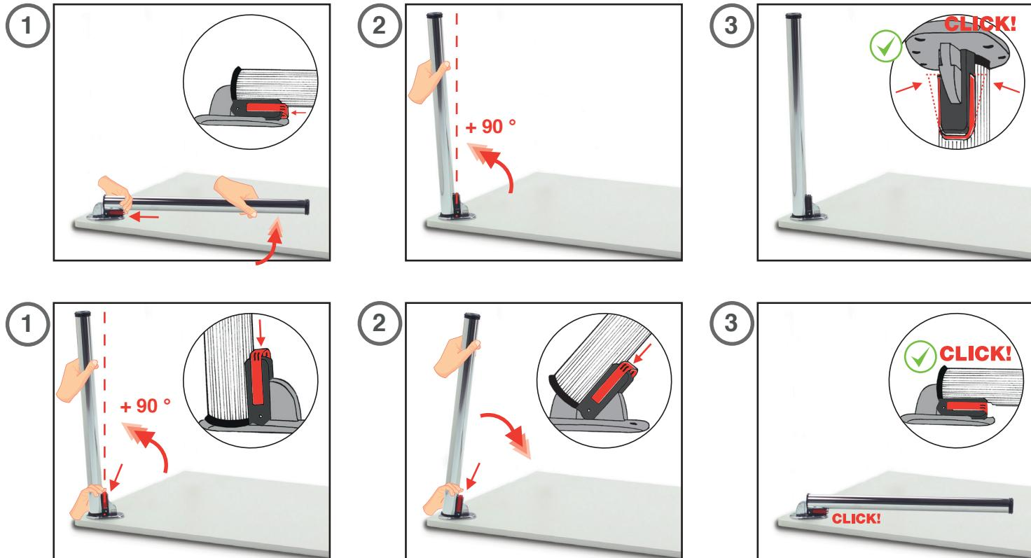
For correct use, open the leg until the safety lock snaps completely.
