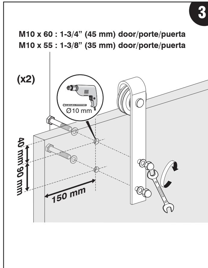
**Step 3: Attach the single bearing supports**
