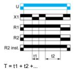
Function: 1 Output with Retrigger / Restart Control
