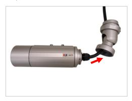
3. Remove the clamping nut and rubber insert to loosen the cable within the gland.
