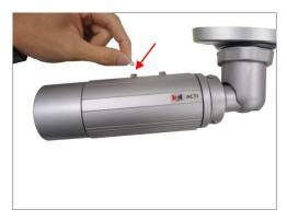
2. Attach the sunshield then loosely secure with the supplied screws.
