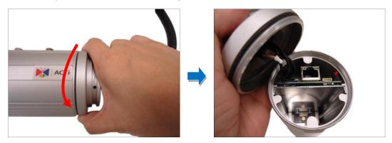
NOTE: Connectors are connected inside the camera, do not abruptly lift the cover.
