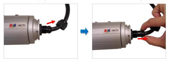
**NOTE:** Connectors are connected inside the camera, be careful when pulling the rubber insert from the gland.
