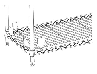
Snap half-sleeve sets onto all four posts at the desired height for the NEXT shelf. Lower this shelf into position and press until fully seated. Install the third and fourth shelves in the same manner, with both shelves mounted ABOVE the post seams.
