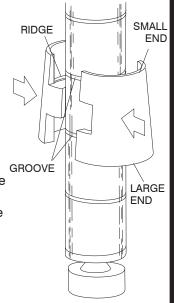
Stand a D Shelf on end, and from the BOTTOM side of the shelf (the bottom side is recessed), slide the TOP end of a post through a corner hole until the half-sleeves are seated in the corner hole. Repeat with remaining posts.
