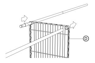
Set the unit upright. Press the shelf firmly at each shelf corner, close to the corner holes, until firmly seated.
