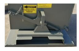
The Hippo Hopper has a single piece gear style rocker designed to allow the hopper to roll forward for a complete dump and then roll back to an upright locked position after dumping (the fewer parts, the fewer problems). Each hopper is also equipped with a pull-down handle, making the hopper easier and safer to dump. Standard finish on all hoppers includes gray industrial paint (optional colors, powder coating, galvanizing steel and stainless steel also available).
