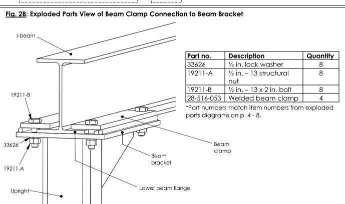
**Step 3:** Tighten the bolts and nuts to 50 - 52 ft·lb using a torque wrench.
