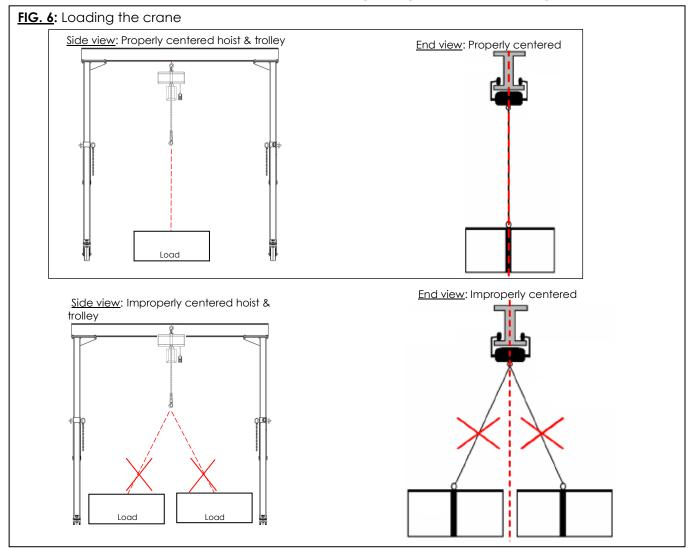
Connect the load to the hoist chain/cable by following the instructions supplied with your hoist and the methods applied at your work site. Then raise the load <u>only</u> as high as is necessary to position it.
