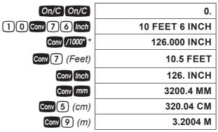
\* Converting a linear value using the **1000**° key will result in the decimal Inch equivalent of the value, rounded to three decimal places. Only unitless values are multiplied by 0.001 Inches when using this key.
