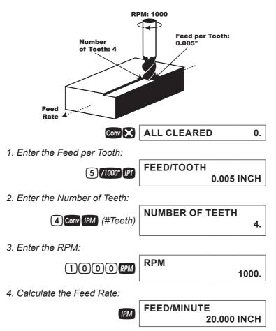
For End Milling (2), find the Feed Rate (IPM) using 1020 Low-Carbon Steel (1) and a 4-Tooth High Speed Steel Tool (1) with a Diameter of 0.5", a 0.25" Width of Cut and a 20" Length of Cut. Then, change the Width of Cut to 0.15" to show the Adjusted Feed per Tooth and the RCT Adjustment Factor. Then, add a 0.125" Depth of Cut and find the Material Removal Rate, Spindle Power and Spindle Torque:
