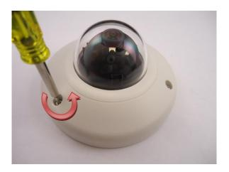
2. Based on the live view from the camera, adjust the viewing angle with pan and tilt direction (for Mini Dome models only).
