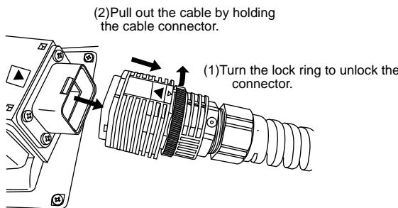
2 Then pull out the cable by holding the cable connector
