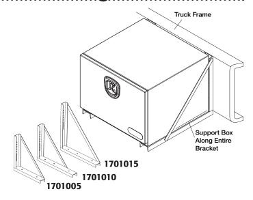
To properly support your Underbody Toolbox, we recommend the use of bottom support mounting brackets. These brackets should be placed so that each end of the toolbox is supported by the full width of the mounting bracket. To prevent water leaks, apply silicone sealant all around each fastener after installation.
