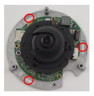
4. Install the camera body to the ceiling using the three (3) screws included in the camera package.
