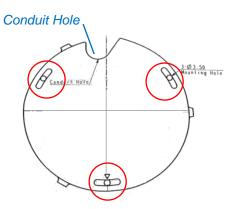
**NOTE:** Depending on the surface where you will install the camera, it may be necessary to drill three (3) holes with  $\phi$  3.5 on the ceiling and use the supplied screw tox.
