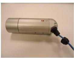
6. Tighten the screws of the back side cover on the camera properly
