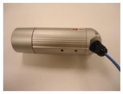
7. Tighten the sealing nut as far as possible.
