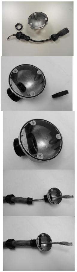
3. Remove the bundled network cable and connector from back side cover of the camera.
