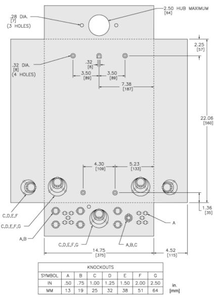
WHEN MONTING THESE LOAD CENTERS, ALLOW 1.25 INCHES OF CLEARANCE ON HINGED SIDE FOR THE DOOR TO OPEN.
